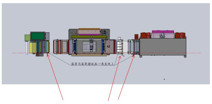
The rollers are arranged in a straight line with each other
